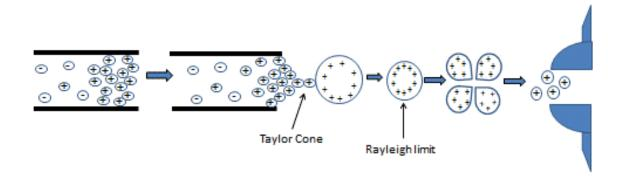
Figure 1: Depiction of ionization by nESI. Reprinted with permission from [Amer et al., 2019].
