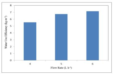
Figure (10): The effect of effluent flow rates on the water use efficiency of tomato plants at the end of growing period.
