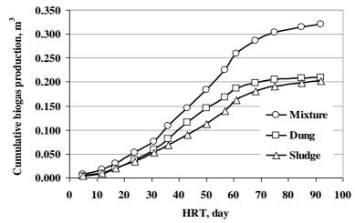
Fig. 2: Cumulative production of biogas during the experiment.
