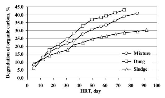
Fig. 5: Degradation of organic carbon for sewage sludge, dung and mixture.
