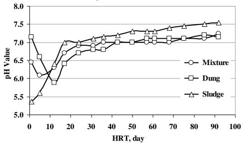
Fig. 4: pH values intervals during the experiment for sewage sludge, cattle dung and mixture.
