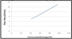
Figure (6): The relationship between consumed energy (E) and its pump speeds (Lit/min).
