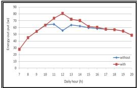
Fig (8): Variation of energy output (E) for PV with cooling and without cooling at daily hours.
