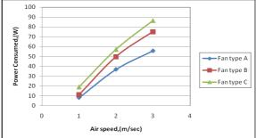
Figure (5): The relationship between power consumed, (W) for three types of fan blades and its air speeds (m/s).
