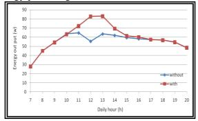
Fig (10): Variation of energy output (E) for PV with cooling and without cooling at daily hours.
