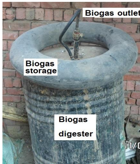
Fig. (4):- Experimental biogas digester
