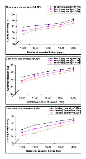
Fig(6): Cutting efficiency at different levels of rotational speed of knives and different levels of dry feeding quantity at the three levels of moisture content for the modified machine.
