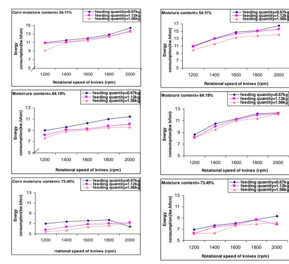
Fig(8): Chopping energy at different levels of rotational speed of knives and different levels of dry feeding quantity at the three levels of moisture content for the modified machine.
