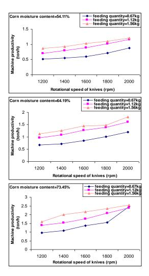
Fig(10): Machine productivity at different levels of rotational speed of knives and different levels of dry feeding quantity at the three levels of moisture content for the modified machine
