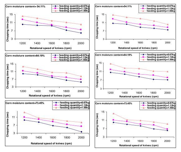
Fig (2): Chopping time at different levels of rotational speed of knives and different levels of dry feeding quantity for modified chopping machine
