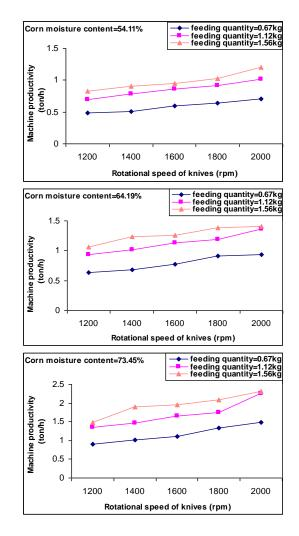
Fig(11): Machine productivity at different levels of rotational speed of knives and different levels of dry feeding quantity at the three levels of moisture content for the non modified machine.
