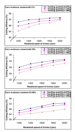
Fig(7): Cutting efficiency at different levels of rotational speed of knives and different levels of dry feeding quantity at the three levels of moisture content for the non modified machine.
