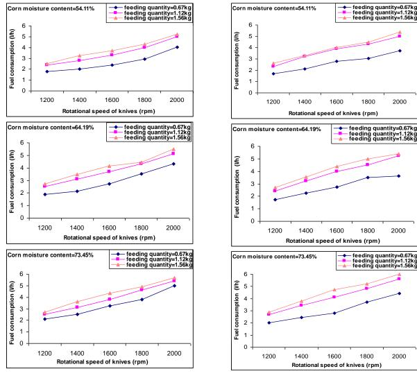
Fig (4): Fuel consumption at different levels of rotational speed of knives and different levels of dry feeding quantity for modified machine
