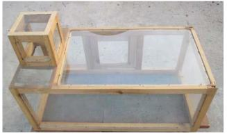
Figure (2): The solar dryer.
