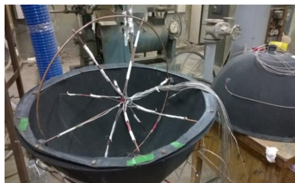
Fig. (2.4) Thermocouples distribution inside the sphere
