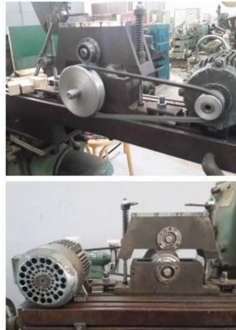
Figure 12. Wear testing machine
