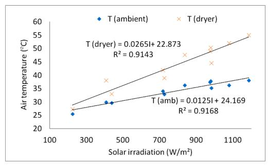
Fig. 4 The relation between solar irradiation and air temperatures (ambient and average value inside the dryers)
