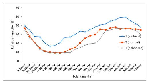
Fig. 3 Air relative humidity VS solar time during experimental drying of tomatoes.
