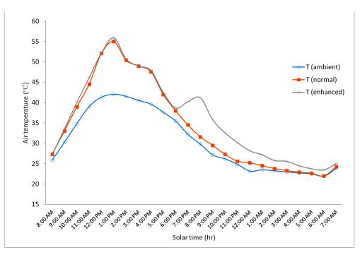
Fig. 2 Air temperature VS solar time during experimental drying of tomatoes.
