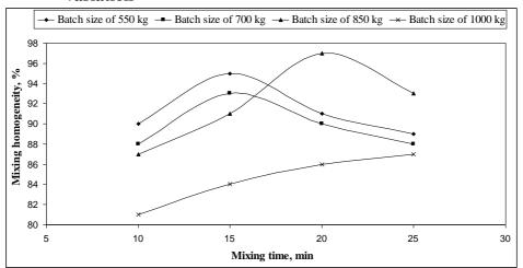
**Fig. (4): Effect of mixing time and batch size on the mixing homogeneity** As to the effect of mixing time on the coefficient of variation and mixing homogeneity at batch size of 1000 kg, results show that increasing mixing time from 10 to 25 min, decreased C.V. values from 15.0 to 10.4 % while increased homogeneity from 81 to 87 %.
