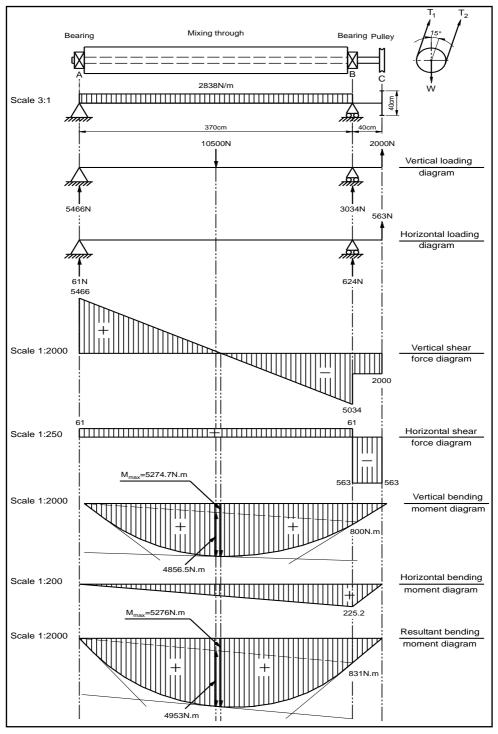
Fig. (2): Resultant bending moment diagram of mixer shaft.
