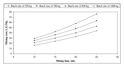
Fig. (7): Effect of mixing time and batch size on mixing cost
