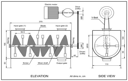
Fig.(1): Schematic views of the developed mixer
