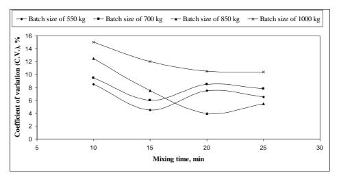
Fig. (3): Effect of mixing time and batch size on coefficient of variation
