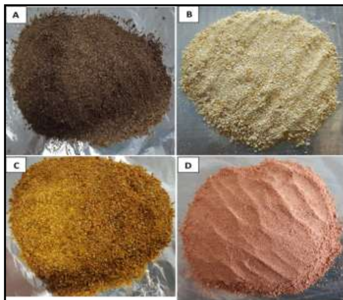
Fig 1: Shapes of grinded dry fruit peels after the mechanical pretreatment; a) banana peels, b) orange peels, c) mango peels and) pomegranate peels.
