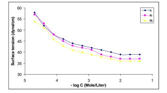
Fig. 3. Surface tension vs. – log concentration of surfactants at (20  $^{\rm o}C).$
