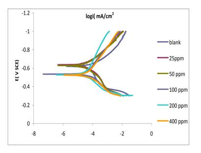
Fig. 7. Anodic and cathodic polarization curves for carbon steel in 1M HCl at different concentrations of IIIb.
