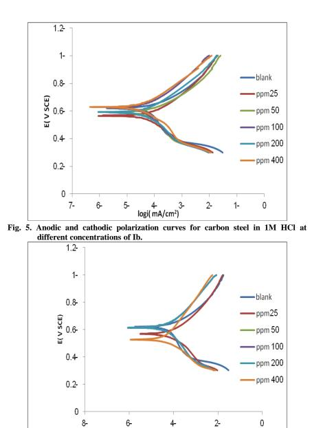
Fig. 6. Anodic and cathodic polarization curves for carbon steel in 1M HCl at different concentrations of IIb.
