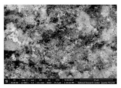
Fig. 7. SEM- unsupported Ni before reduction of p- nitrophenol.
