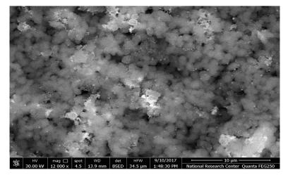
Fig. 9. SEM - Ni/ Zeolite before reduction of p-nitrophenol.
