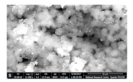
Fig. 10. SEM- Ni/ Zeolite after reduction of p-nitro phenol.
