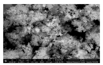
Fig. 8. SEM -unsupported Ni after reduction of p-nitrophenol.
