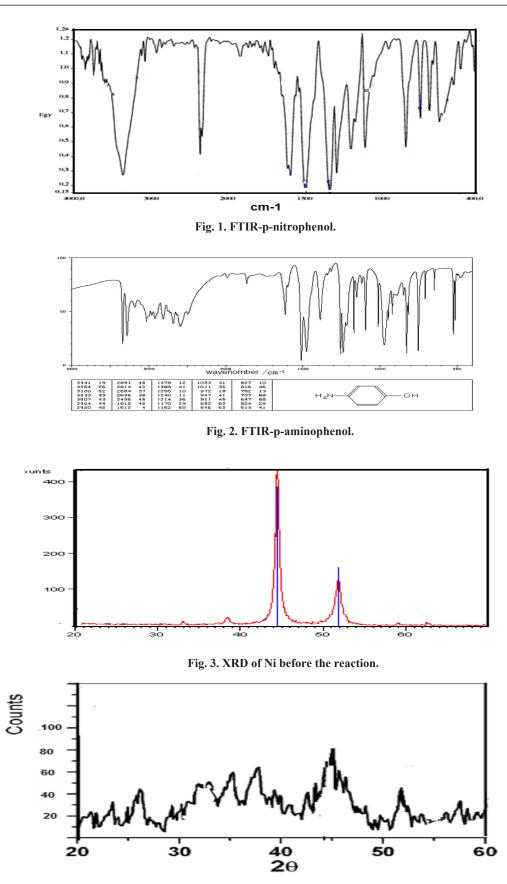
Fig. 4. XRD of Ni after the reaction.
