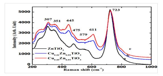
Fig. 2. Raman shift of thin films (a) ZnTiO<sub>3</sub> doped with two different concentrations of Cu ions (b)1 and (c) 5 mol% deposited on quartz substrates and annealed at 600 °C for 1 h.
