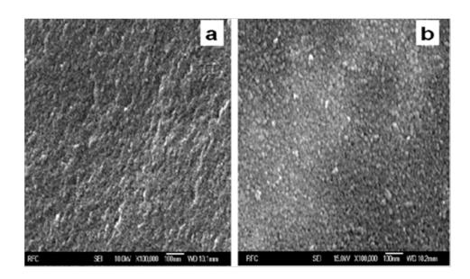
Fig. 3. FE-SEM images of the ZnTiO<sub>3</sub> and Zn<sub>0.95</sub>Cu<sub>0.05</sub>TiO<sub>3</sub> thin films deposited on quartz substrates and annealed at 600°C for 1 h.
