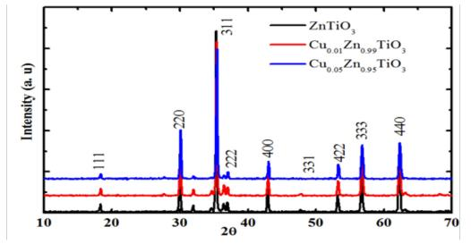
Fig. 1. XRD pattern of Zn<sub>1-x</sub>Cu<sub>x</sub>TiO<sub>3</sub> (x = 0%, 1%, 5%) thin films deposited on quartz substrates, annealed at 600 °C for 1 h.
