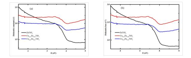
Fig. 6. (a) Real part, (b) Imaginary part of dielectric constant as a function of photon energy for  $ZnTiO_3$ ,  $Cu_{0.01}Zn_{0.99}TiO_3$ , and  $Cu_{0.05}Zn_{0.95}TiO_3$  thin films.
