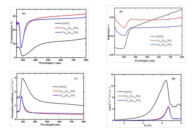
Fig. 4. (a) Transmittance, (b) Reflectance, and (c) Absorption coefficient as functions of wavelength. (d)  $(\alpha hv)^2$  as a function of photon energy for ZnTiO<sub>3</sub>, Zn<sub>0.99</sub>Cu<sub>0.01</sub>TiO<sub>3</sub> and Zn<sub>0.95</sub>Cu<sub>0.05</sub>TiO<sub>3</sub> thin films with thickness 250, 276 and 300 nm, respectively, deposited on glass substrates and annealed at 400 °C for 1 h.
