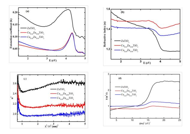
Fig. 5. (a) Extinction coefficient and (b) Refractive index as functions of wavelength. (c)  $n^2$  as a function of square wavelength. (d)  $1/(n-1)^2$  as a function of square photon energy for  $ZnTiO_3$ ,  $Cu_{0.01}Zn_{0.99}TiO_3$  and  $Cu_{0.05}Zn_{0.95}TiO_3$  thin films with thickness 250, 276, and 300 nm, respectively, deposited on glass substrates and annealed at 400 °C for 1 h.
