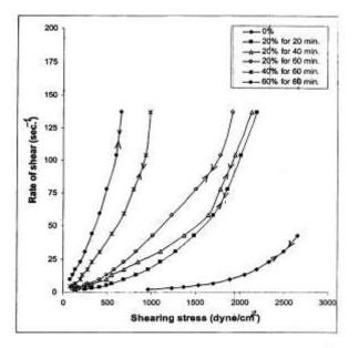
Fig. 4. Effect of urea concentration & reaction time on the apparent viscosity of carbamated fenugreek galactomannan gum (6%) treated with NaOH (1%) at different rates of shear (after 24 hr storing).
