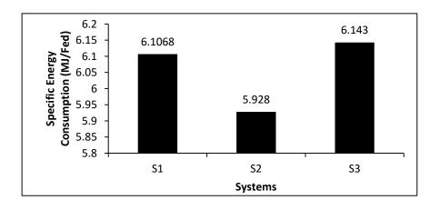
Fig. 5. Specific energy consumption of different tillage.
