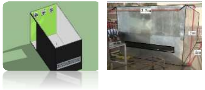
Figure 2: Design of the poultry house
