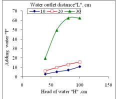
Fig. 11: Effect of head of water H", cm on adding water at different water outlet distance, buried depths (10 cm), sensor volume (25cm<sup>3</sup>) and rubber thickness (3.5 cm)
