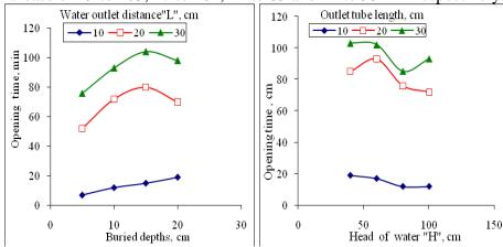
Fig. 14: Effect of buried depths on opening time at different water outlet distance, sensor volume (25 cm<sup>3</sup>), Head of water (100 cm), and rubber thickness (3.5 cm)
