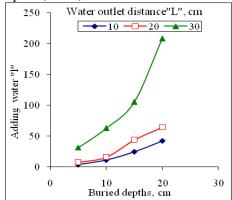
Fig.10: Effect of buried depths on adding water at different water outlet distance head of water (100 cm), sensor volume (25cm<sup>3</sup>) and rubber thickness (3.5 cm)
