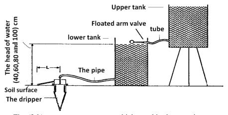
Fig. (2-b) apparatus component which used in the experiments
