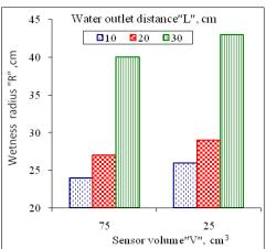
Fig. 5: Effect of sensor volume on wetness radius at different water outlet distance, Head of water (100 cm), buried depths (10cm) and rubber thickness (3.5 cm)
