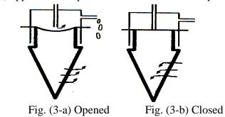
Fig. (3) Schematic diagram of self control dripper work
