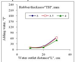
Fig 8: Effect of water outlet distance on adding water at different rubber thickness, head of water (100 cm), sensor volume (25cm<sup>3</sup>) and buried depths (10cm)
