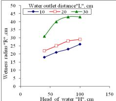
Fig. 6: Effect of buried depths on wetness radius at different water outlet distance, Head of water (100 cm), sensor volume (25cm³) and rubber thickness (3.5 cm)
