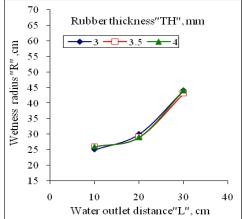
Fig. 4: Effect of water outlet distance on wetness radius at different rubber thickness,head of water (100 cm), buried depths (10cm)and sensor volume (25cm<sup>3</sup>)
