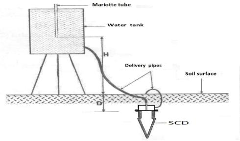
Fig. (2-a) apparatus used in the experiments
