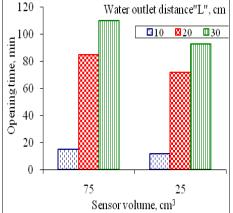
Fig. 12: Effect of water outlet distance on opening time at different rubber thickness, Head of water (100cm), buried depths (10cm) and sensor volume (25 cm<sup>3</sup>)
