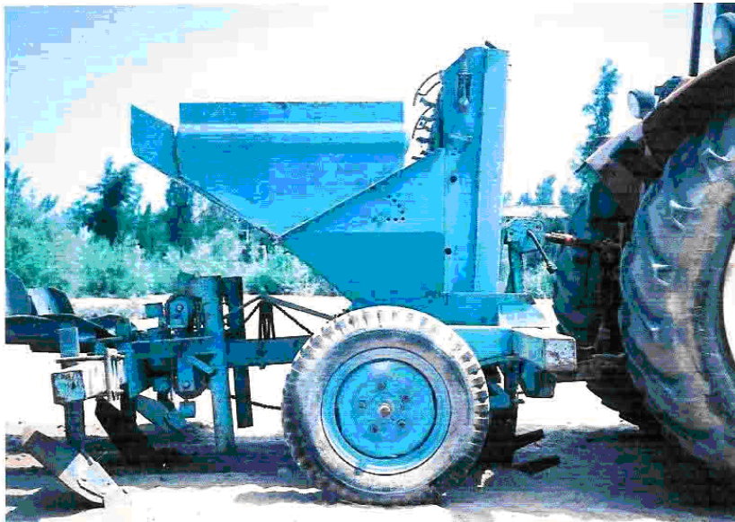
Fig.(1): photography view of the potato planter.
