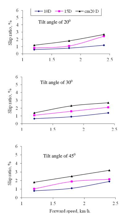
Fig. 9: Effect of forward and compressed wheel depth (D) on tractor wheel slip under different tilt angles, degrees for surface mulch
