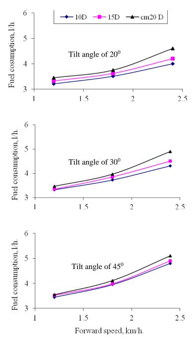
Fig. 10: Effect of forward speed and compressed wheel depth (D) on fuel consumption under different tilt angles for subsurface mulch
