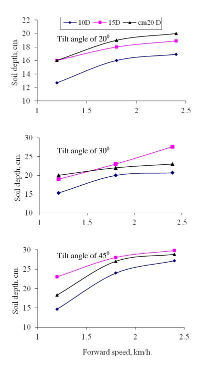
Fig. 7: Effect of forward speeds and compressing-wheel depth (D) on soil covering depth under different tilt angles for subsurface mulch
