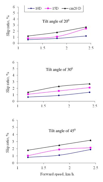
Fig. 8: Effect of forward speed and compressing-wheel depth, (D) on tractor wheel slip under different tilt angles for subsurface mulch
