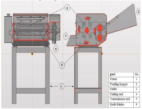
Figure (1): Developed disc-chopper views
