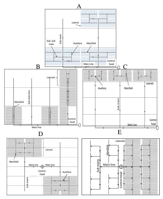
Fig (1): Layout pattern from "A" to "E" that the model investigated.
