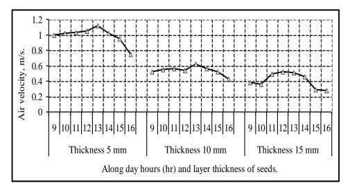
Figs. 6: Effect of drying time, layer cucumber seeds thickness on the air velocity.
