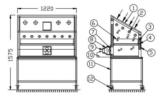
Fig. 1: Elevation and side views for the cabinet dryer.
