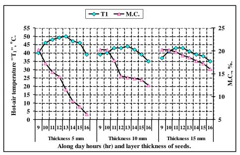
Fig. 7: Effect of drying time, layer thickness of cucumber seeds and drying hot-air temperature " $T_1$ " on moisture content "M.C.".
