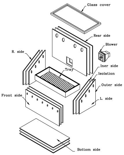
Fig. 2: Isometric and parts of the cabinet dryer.
