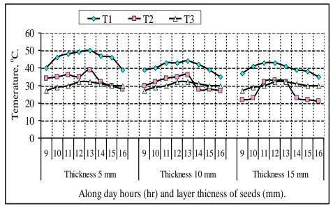
Fig. 4: Effect of drying time and layer thickness of cucumber seeds on the temperature ( $T_1$ : hot-air temperature,  $T_2$ : cucumber seeds temperature and  $T_3$ : ambient temperature).
