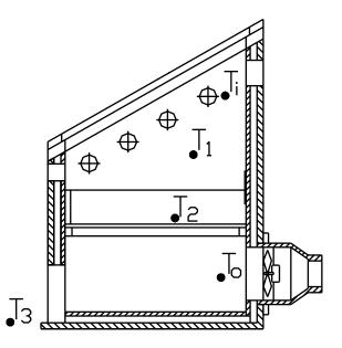
Fig. 3: Distribution of 5 thermocouple points inside and outside drying box.
