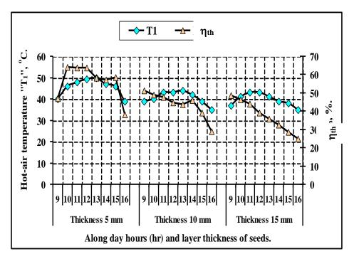
Fig. 8: Effect of drying time, layer thickness of cucumber seeds and drying hot-air temperature "T1" on the thermal efficiency " $\eta_{th}$ "
